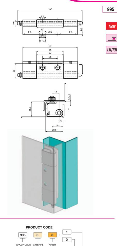
Side part can be mounted with M 5 screws.
